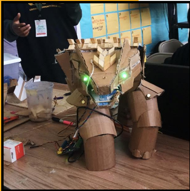
Ankylosaurus robot with programmed light sensor, LED's and servo-motor by Makei and Nicolas.
